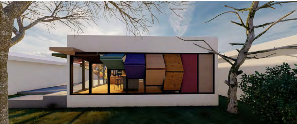
Figure 96 The shading devices made from reclaimed doors are half open, half closed.
