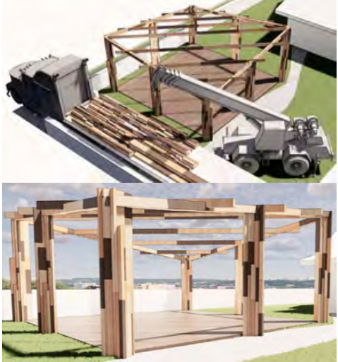
Figure 103 Assembly process of the post and beam structure
